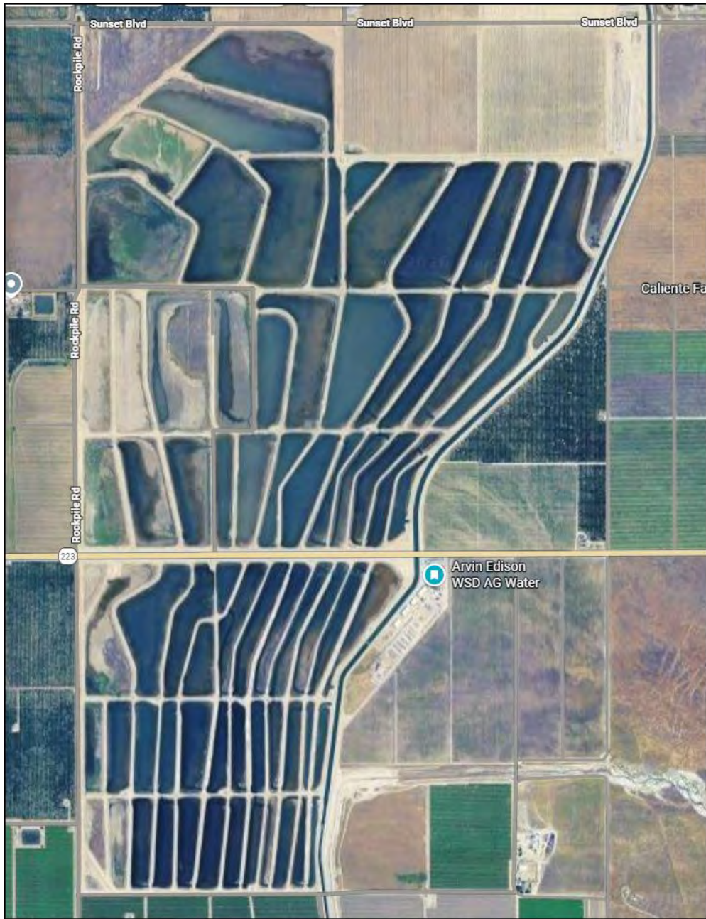
Figure 3. Aerial image of the Sycamore Spreading Works, an Arvin-Edison Water Storage District facility, an example of what the final layout may look like for a large recharge basin facility.
